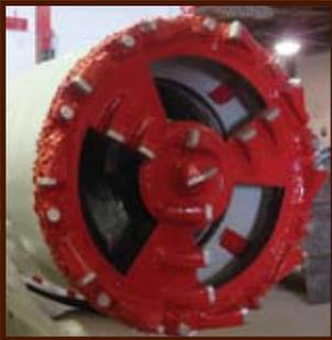
*Front Steer Boring Unit (FSBU) with open face cutting wheel.*
