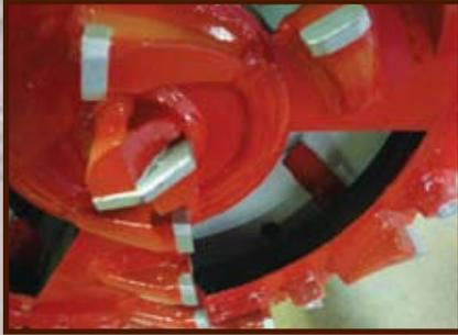
*Two high pressure water jets are located on the bottom side of the open face cutting wheel to ease the movement of material through the system.*
