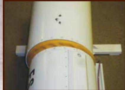
*Hydraulic fluid is sent to the FSBU and causes an articulated movement which instantly makes corrections to the intended Line and Grade.*
