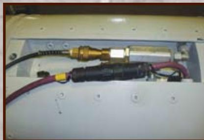
*Connections for hydraulic and electric to the FSBU, which is protected by a steel cover plate (not shown), are conveniently located at the back of the unit.*
