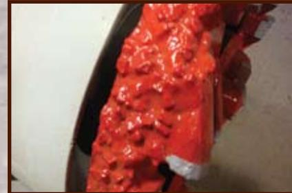
*A specially hardened cutting edge helps excavate and maintain overcut in harder soil conditions.*
