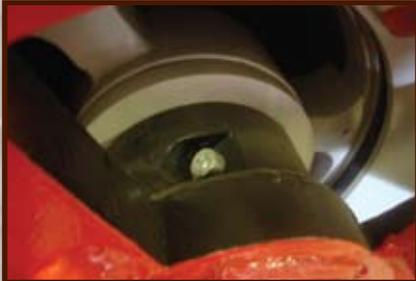
*The open face cutting wheel can be removed and unbolted for maintenance and insertion of the illuminated LED Target.*
